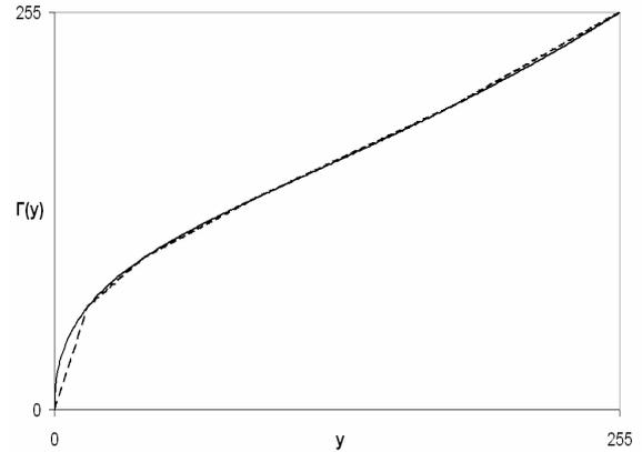
**Figure 4.  $\Gamma$  transformation (straight line) and its piecewise linear approximation (dashed line)**
