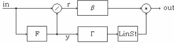
Figure 1. Block diagram of Retinex-based operators
