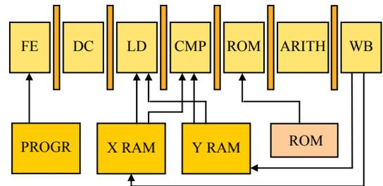
**Figure 5. Pipeline structure and memory accesses**
