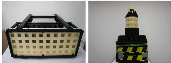
Fig. 3. Antenna array at the BS (left) and at the MT (right).
