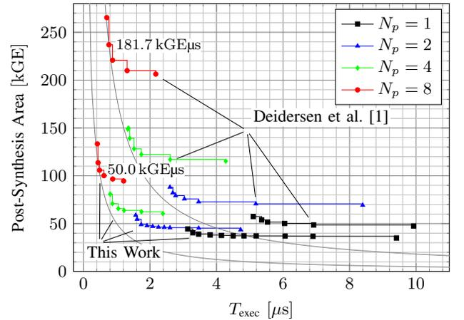
Fig. 6. Area vs. execution time based on the MCMC detector's synthesis results, comparing this work to [1], assuming  $N_t = 4$ ,  $K = 6$ .
