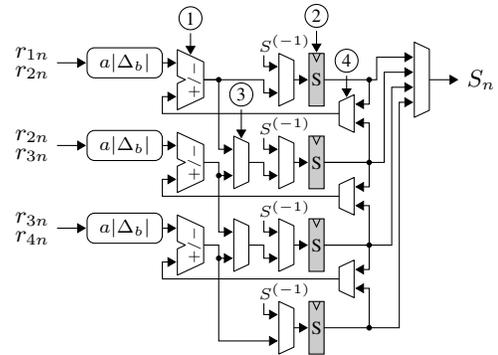
Fig. 4. Update-S-Circuit. Example for  $N_t = 4$  antennas. All units exist for the real and for the imaginary parts respectively (not drawn).
