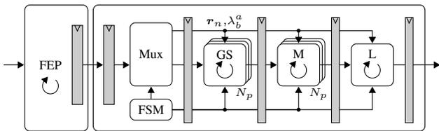
Fig. 2. Architecture design of the MCMC detector. The  $n$ -th column  $r_n$  of  $\mathbf{R}$  and  $\lambda_b^a$  are selected in the Mux stage. FEP and MCMC core computations overlap thanks to double buffering.
