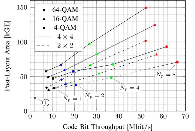
Fig. 7. Area vs. throughput based on the MCMC detector’s layout results. For each design-time configuration, the ASIC with the fastest clock is shown. As an example, the 16-QAM  $2 \times 2$  design supports one or two antennas and 4- or 16-QAM at run-time.
