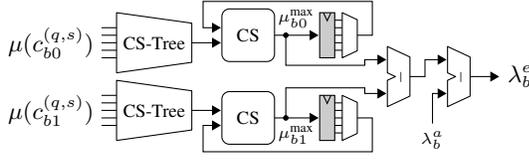
Fig. 5. L-Circuit. Data tokens propagate alongside the data values. The registers hold tokens and values. The Compare Select (CS) elements forward the data item with the larger value if both are valid.
