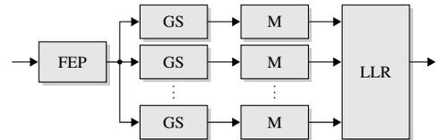
Fig. 1. Partitioning of the low-level algorithm: Front-end Processing, Gibbs Sampler, Metric Update, LLR Computation.
